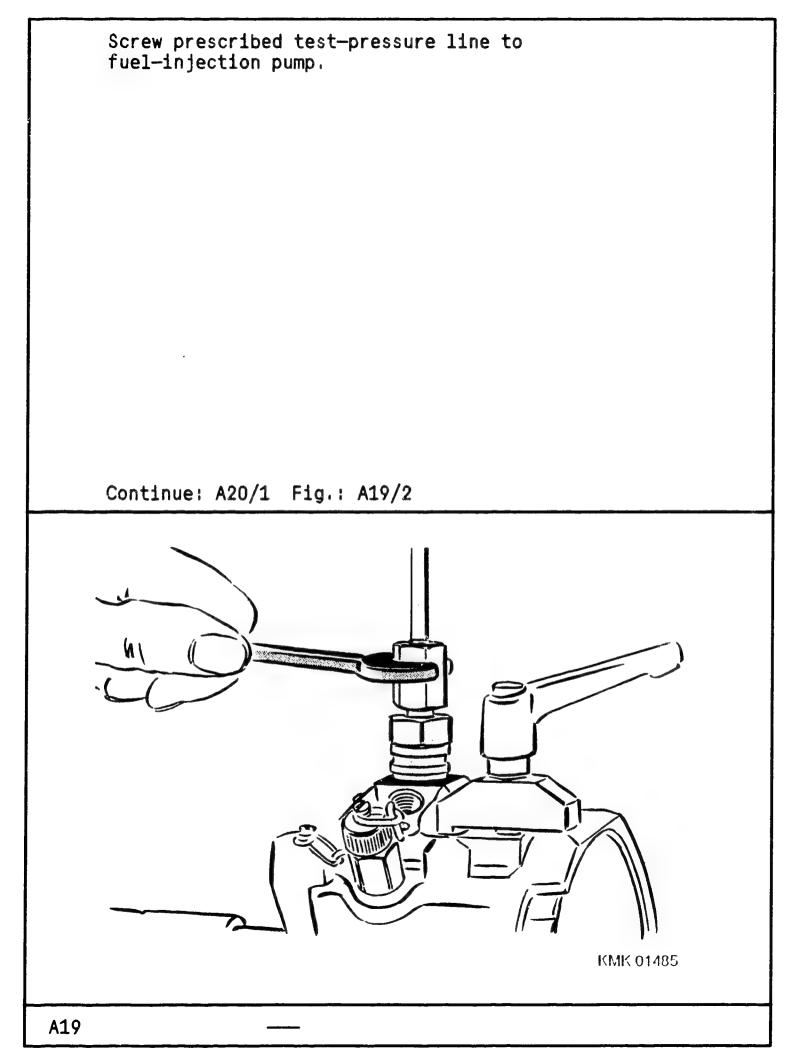
Assemble test-pressure lines vertically on delivery-valve holder and calibrating nozzle-holder assembly.
